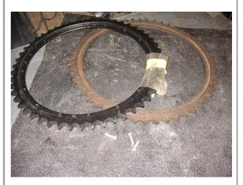
I know that you change the front sprocket when you replace the chain. I would like to say I do the rear sprocket too, but I usually just run it. You can buy a whole drum and sprocket assembly aftermarket. If you do want to rivet on the sprocket, here are two of them. Note the loose rivets in front. They fell our of the little bag. This is why I like plastic tubs instead of cardboard boxes. Those tiny parts can't leak out of a tub.
