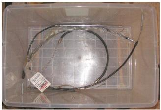
At the bottom I put an early model front brake cable with a nice chrome tube. Also a rear brake cable like on the 1975-6, and a front brake hydraulic line. I consider the rear brake cable death hardware. I have had nothing but trouble with them, whether the 1975-6 external cable or the 1977 internal one.
