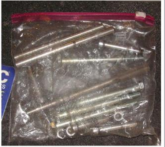
I remove the Mickey Mouse pins on the 1978-83 dual front calipers. Then I install pieces of drill rod and use a set screw to hold them in the fork tubes. I have a reamer back-ground by Charlie Jackson so I can hog out the calipers so the drill rod fits perfectly. This stabilizes the calipers, stops them rattling and makes them stop much better. I will write up a detailed guide now that I live in beautiful Florida and have time to document these things.
