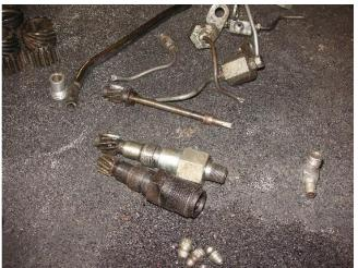
The tach drive goes in the gearcase tub, the speedo drive went into the gauge tub.
