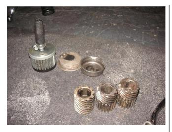
I have no idea why crankshaft gears were in this tub, I will put them in the right place. In back you can see some breather stuff. That should have gone into the gearcase tub, that where I will put them.
