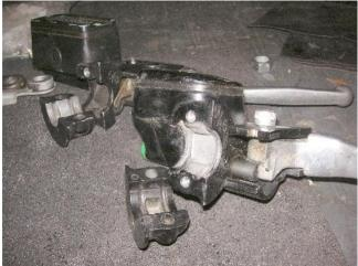
You can make the older front master cylinders work, but the late-model master cylinder have bigger reservoirs and better levers. You can buy them cheap. These are destined for my 1977 and 1980 show bike. I have already replaced the master cylinder on my 1979. The 1977 has an old factory setup an the 1980 has the dreaded Arlen Ness master cylinder. The only brakes I can vouch for are GMA, since those are on my 1983 XR-1000 and it stops like it has retro-rockets.
