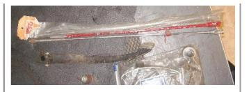
So help me, as little as you use the rear brake, I would make all my bikes mechanical if I could. Here are three rear brake rods, all different lengths, since there are at least two different length swingarms. Also and early brake pedal and spring. That is a good candidate for eBay.
