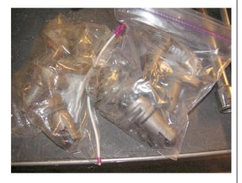
I have two complete sets of the cast iron lifters from early Sportsters. I figure they have to last longer than the aluminum ones. I do get way more life out of the aluminum ones after Duncan Keller taught me to blow off the lifer and corks before adjusting the lifters. That way no grit and dirt falls into the lifters and they don't get all scored and worn out.
