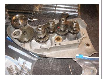
Here is the gearcase with a set of cams. Note that high-zoot drilled-out idler gear given to me by Roger Reed.
