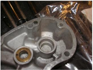
I think the 1969 gearcase cover uses the pressed-in flange. The early covers have a spring-loaded flange that presses against the large washer on the generator. Engine breathing was always a little funky on Sportsters, until 1977 when it got so cost-reduced it the engine stopped breathing at all.
