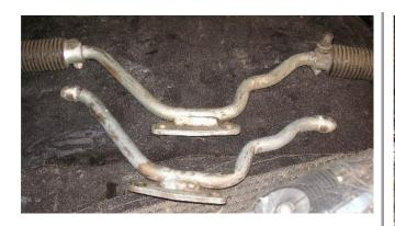
Here are two early model rear footpeg mounts. I run these whenever I can. Its much better for your passenger to have the pegs bolt to the frame instead of the rear swingarm like some later models. You also have to run the spring on at least the right one so it will always stay up out of the kickstarter's way. Only the finest women make sure to pull up the right peg after they get off the bike. I will be keeping my eye our for such a gal out here.
