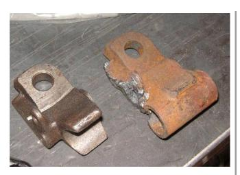
When the kickstand mount gets egged out since you put a 16-inch wheel on the back of your 1977 kick-only Sportster, and a 21-inch wheel on the front, you can weld in a piece cut from an old frame, or the factory made repair sections like on the left. Priceless.
