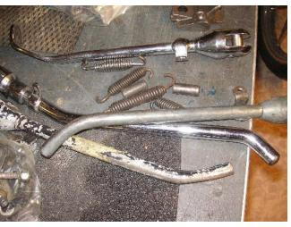
There are four kickstands, or sidestands, if you prefer. Some springs and a pin. The aftermarket stand with the pinch bolt is junk, especially if the pinch bolt peens over the metal and you cant get the dang kickstand off the bike. The stock pin setup works, if you set it up right and bend the stand so the pin does not take too much pressure.
