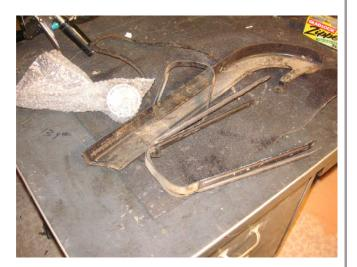
Also in the tub was the K-Model chain guard, and some fender struts. The trick is to take early Sportster struts and rivet them to a Hummer front fender. The Hummer fender is the same as K-Model, with the little flip at the back.
