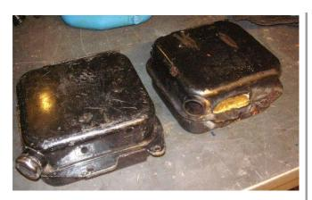
Here are two "lunchbox" oil bags from the 1970s. Note one is patched up with brazing. That can really backfire— the brass gets into the steel and the tank will crack for eternity. Kenny Puccio tells me that modern thinking is to weld the leaks. Fix the steel with steel. The reason for the brazing will soon be obvious.
