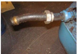
Here is a crappy pic of the k-model oil feed line. The tank had the fittings on it, so that is what you look for in these early tanks. The later model tank will fit, but not have the fittings on the tank or motor.
