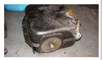
The brazed tank I have modified to mount an oil filter. This is a pretty high-zoot modification. There is a pipe also brazed on the inside to feed the filter from the existing feed hole. I can't remember if I ran this one or if it just leaked as I kept chasing cracks with brazing rod. Don't laugh, I run a similar mod on my 1977 and it has worked for years. I am pretty sure that one is brazed up as well.I think I wanted a chrome one on the '77. This one might work fine, I will test it for leaks.
