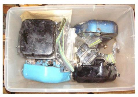
The oil tub is one of the lighter tubs on the Gorrlla rack shelving. Here you can see the two kidney style oil bags as well as an XLCH style "lunchbox" oil tank. Also an early coil cover. The bottom of the tub has oil pumps and fittings and filter mounts.
