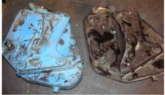
Here is the backsides of the K-model oil tanks. The fact that they have threaded fittings for all the oil lines makes them very early production. I love to note the minor differences in the mounting brackets and other features on the tanks.
