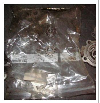
Little things can be valuable, here are some oil pump gears for pre-1977 Sportsters. Note the spring at bottom for ealry model check ball setups. I am trying to keep my 1962 from sumping.
