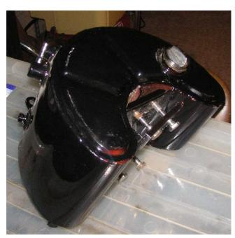
This gorgeous baby was in the spare room, so I am adding it to the oil tub. It is a restored horseshoe-style Sportster oil tank used on XLCH models. There are some part numbers for this tank with a -52 suffix, so I suspect it was created for the racing K-Models, the overhead-valve Sportster came out in 1957.
