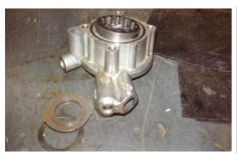
Here is a big-bike pump with larger gerotors. My plan is to make a housing that holds this set of gerotors where the generator mounts to the case. Then I can scavenge the motor there, and keep a negative pressure in the crankcase like there should be.
