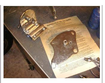
Most kick-start Iron Sportsters don't have an oil filter. I have to think the Harley engineers thought the weight was so critical or that they would leak so much we could get by without a filter. Here are two after-market filter setups, or maybe the frame-rail one is a factory setup, not sure. The funky plate replaces the motor mount and you run long hoses to the filter. This is why I hacked that lunchbox oil bag, less hoses and fittings are less places to leak.
