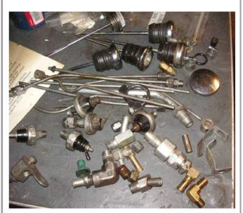
Here are all the dipsticks, oil-pressure switches, and small stuff in the oil tub.
