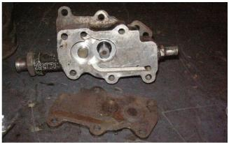
Here is a pre-1977 pump, with the wide slot so it is for 1000cc bikes after 1972. Best thing was the pump had the spring and ball bearing so that I might be able to keep my 1962 from sumping when it sits for a month.
