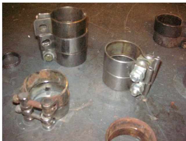
Some wider clamps used on the normal diameter pipes. The 1970 clamps look similar, but they are for a much smaller pipe.
