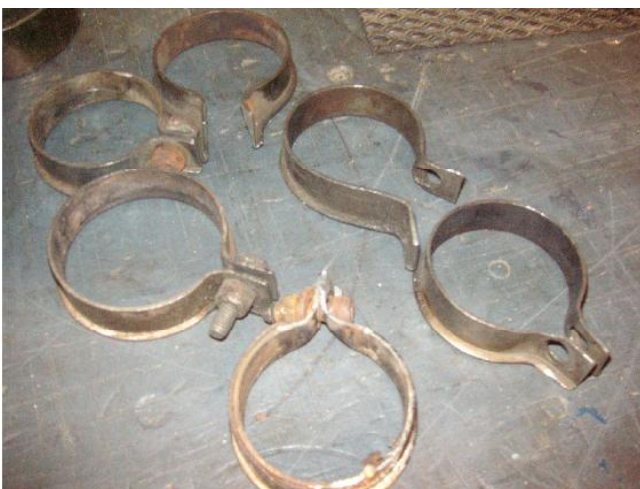
Some old factory clamps in thin sheet metal with the flange to give structure.
