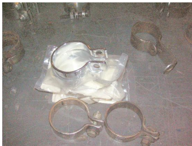
Here are some factory clamps, some new in the bag that they used on the pipe at the head. Sorry, I will get the part numbers next time I am in the tub.
