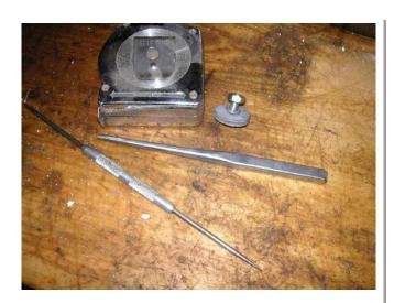
Here are the main tools. A dental tool pokes a hole in the tarp, the drift opens the hole up. Ruler is to get the two sides level.
