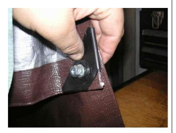
The 1/4-20 bolts pass through a grommet and a hole you punch in the other side. I ran out of fender washers so this side just has an SAE washer.
