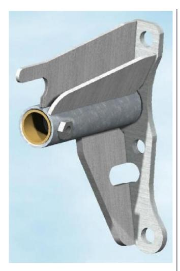
So without having to scrap a weldment, I could sit and look at the screen and try to figure out the cleanest way to provide clear access to the stud nuts and still anchor the return spring.
