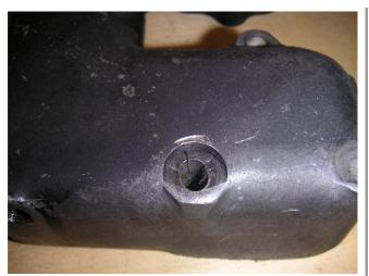
And once again, paper is just part of it. Keep riding and you realize why it is bad to make the rocker boxes into the top motor mount like Harley did in 1977. When other mounts get loose, you end up with this. And this is only when things go really wrong. The rocker box gaskets start leaking long before this stage of destruction. Maybe those old-time Harley engineers tied the top mount to the heads for a reason.
