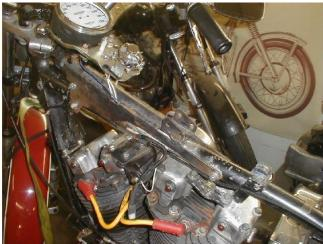
I was reluctant to weld on my frame. I splatter more than I weld. Just sitting next to the bike and playing with the mount, I realized I could weld side-plates to the aftermarket mount, and then bolt the whole thing to the frame.
