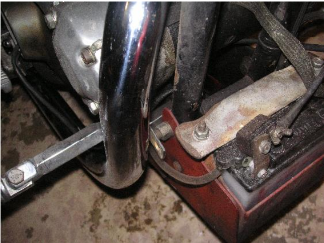
You can just make out the tab where it lines up to the motor mount bolt.
