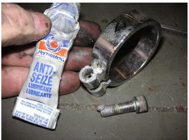
Anti-seize on the bolt threads and where the head runs on the clamp.
