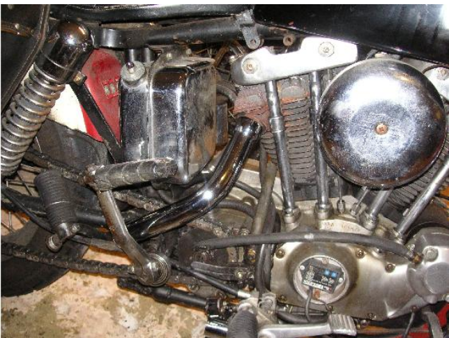
Trial fitting of the rear pipe. So far so good.
