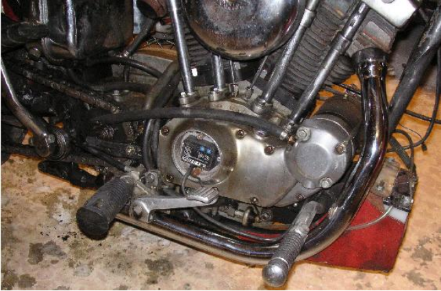
Trial fitting of the front pipe.
