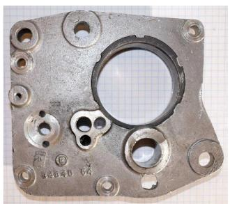
The same 34845-54 casting number as the K-model door, but a different casting at the primary boss mount.
