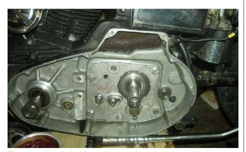
The trap door is held in with 4 5/16 course-thread bolts on the left side of the engine. (courtesy scottericsonon)
