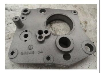
The 1952 and 1953 K-models did not have a trap door. You have to split the cases to service the tranny. The 1954 door is similar to the -57 door but the dowel holes are tapered, instead of straight. The boss to mount the primary cover sticks out much further.
