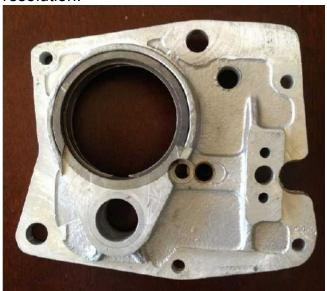
The increased material beteen the shaft bearings is a good feature of this part, and why you might want to retrofit it to any 1957 or later bike that does not need the center hole primary cover mount.
