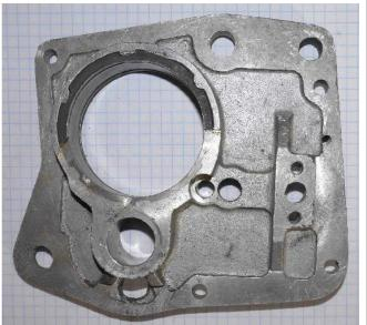
The door is machined for straight dowel pins, otherwise similar to the K-model door. Shorter boss for mounting the primary cover. Shorter boss would allow more parts to fit in a box, but would also strip out easier.
