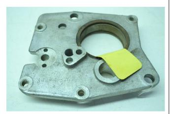
Casting number 34846-76. I think the snap rings in the bearing bore are wider in the 79-later tranny, otherwise identical.
