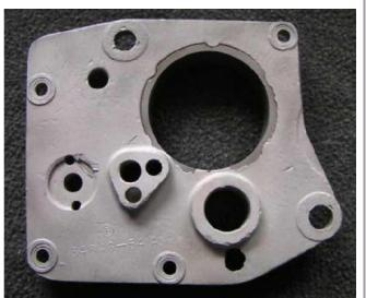
Here the factory bumped the casting number to 34846-54A and removed the boss for the primary cover mount completely. No record of a service part number, this may be a -57A but that number does not appear in the parts books, it is just supposition.
