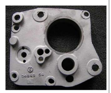
The same 34845-54 casting number which seems correct. The 1/4-20 hole for the primary cover is not drilled. This may have been used on XLCH models that don't use the center-mount primary cover.
