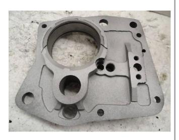
The backside of the trap door is where the shifter mechanism, as well as hte shifter forks, and the gear shafts. Harley engineers must have considered this door part of the left case, hence no part number was cut.
