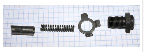
The Sportster shifter cam follower assembly. The 34065-52 cam holder is on the far right. the part numbers from left to right: 34062-52, 34068-52A, 34067-52, 34065-52.
