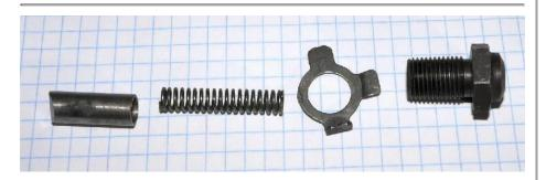
The Sportster shifter cam follower assembly. The 34065-52 cam holder is on the far right. the part numbers from left to right: 34062-52, 34068-52A, 34067-52, 34065-52.
