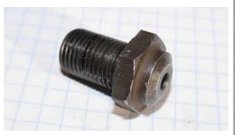
You don't need to torque this very hard, since it has a metal lock tab to keep the bolt from backing out.
