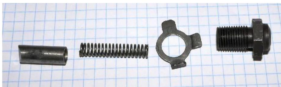
The Sportster shifter cam follower assembly. The 34065-52 cam holder is on the far right. the part numbers from left to right: 34062-52, 34068-52A, 34067-52, 34065-52.
