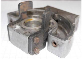
Here is the upper lifter installed and staked on with the two lifter dowel pins.
