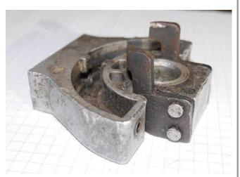
Here is the lower lifter installed and staked on with the two lifter dowel pins.
