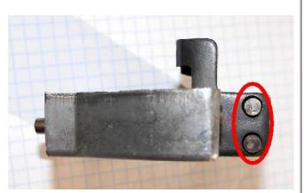
Here is an on-end view of the shifter lifter dowels as installed on the shifter support. The steel parts are called lifters since they lift off the shifter pawls so you can ratchet the carrier both ways.
