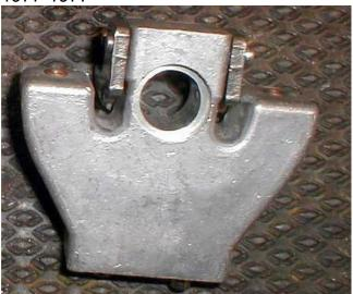
This part revision is for the left-hand shift case redesign in 1977. There is a pocket where the shifter cam plate mounts, since the shifter shaft has to pass right by it.
