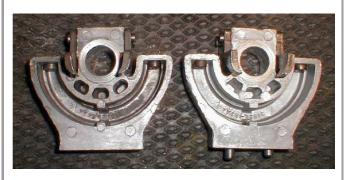
The 34012-52C on the left and the 34012-75 on the right. The pocket in the shaft hole in the -75 part means the shifter cam plate is shorter, as is likely the pawl carrier.
