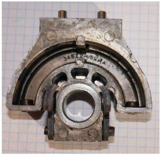
Flipping the part shows where the factory put the casting part number on this die casting. The 34512-52A, while not dispositive, as the lawyers would say, does tend to correlate with the upgrade from the -52 sand-cast part. The letter suffix usually means that this part will retrofit to the older part.
