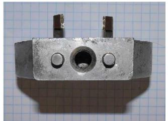
The left-facing mounting surface holds the two locating dowels and has the threaded hole to mount the assembly to the trap door.
