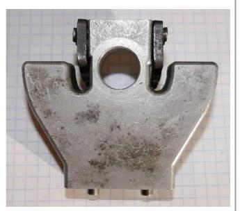
The later parts were die cast. The surface finish and fine detail indicates this is made form zinc, not aluminum. This holder has the "lifters" as well as the two dowels that hold them in, and the two locating dowels on the bottom.
