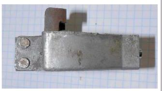
This top view, as it would sit in your bike, shows the two dowel pins for the lifters. You can see the upper lifter and one of the mounting dowel pins as well.
