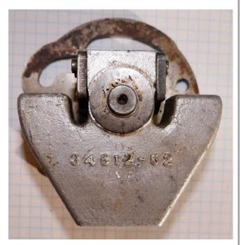
The 34512-52 casting part number on the font-facing side of the holder. The silvery appearance and surface finish of later holders leads me to believe these are zinc, aka pot metal. This part looks sand cast.
