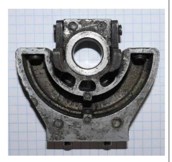
The rear-facing side of the shifter support. In addition to having the "lifters" the lifter dowels, and the locating dowels, this part has the "plugs" at the top of the big grooves, which locate the large return springs that center your shifter lever.
