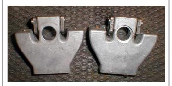
Here is a comparison of the right-side and left-side shifter designs. The 34012-52C on the left and the 34012-75 on the right.
