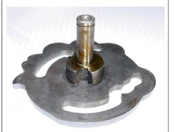
The -52C plates have a big chunk missing from the shaft collar. This may be a function of the upsetting or forging operation, it is hard to believe Harley engineers were just trying to save a few pennies of steel. Its a puzzlement.
