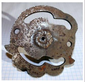
The early plate has two located holes probably used during manufacturing. The weld of the plate to the shaft is uniform and circles the entire shaft.
