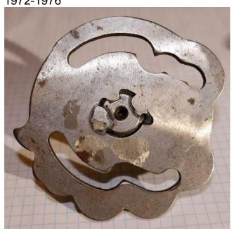
The -52C plate is cost-reduced, being made from a single press blanking operation. Note the rounded edges compared to the early plate. The full-circumference weld is replaced by two tack-welds. One of the "ears" disappears, not sure why.
