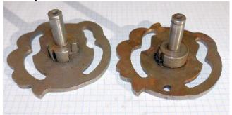
The earlier version on the right has sharper edges, and no chunk missing from the shaft collar. Later part also lacks the two locating holes.
