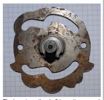
The boss in on the shaft is continuous and there are two "ears" where the detent cam runs. Here detents are 4th, 3rd, 2nd, neutral and 1st from left to right.
