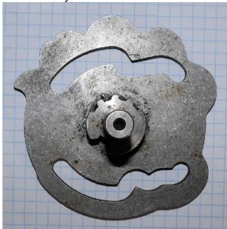
Backside shows shaft has a chunk missing.
