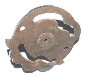
A 3/4 view shows the diligent welding and the sharp edges of this early shifter cam plate.
