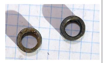
The late-model shifter carrier design uses these spacers in conjunction with flipping the pawl hooks over so they can use the same part for the left and right pawl function.
