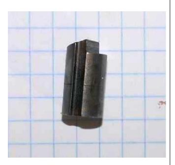
This plunger is the mate to the left one, It ratchets the shifter plate around, which moves the shift forks. There is no part for the 1972 design since that design uses two identical parts that are covered in the Shifter Pawl Left part page.
