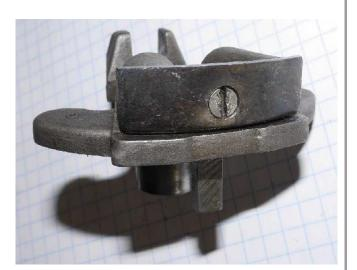
This metal plate retains the pawl plungers and provides a base for the pawl springs to react against. The part number only appears in 1970, althought the part was used since 1952. It is likely Harley considered it part of the carrier.
