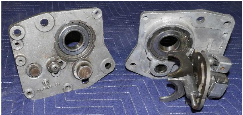
The Iron Sportster trap door assembly holds the mainshaft, countershaft, and shifter mechanism.
