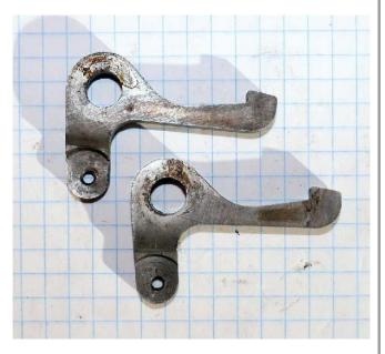
Here is the backside of the late-model shifter pawls.
