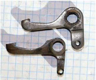
The pawl above is from later production of the part. It has much more metal where the spring attaches.
