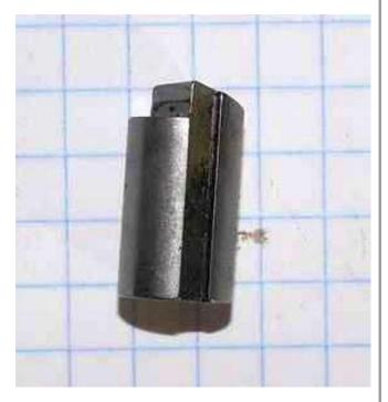
The little slot picks up a pin so this pawl does not rotate. A spring fits inside to press it against the cam plate.
