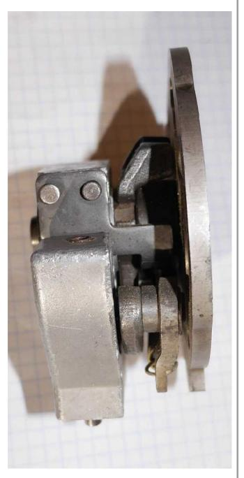
This later version has larger-diameter material on the hooks where they mount to the carrier.
