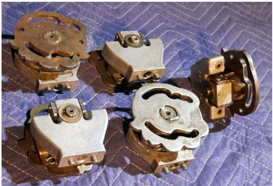
The Iron Sportster shifter comes as the 34009-52 assembly.
