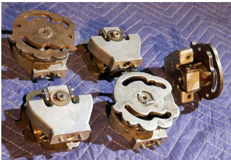
The Iron Sportster shifter comes as the 34009-52 assembly.
