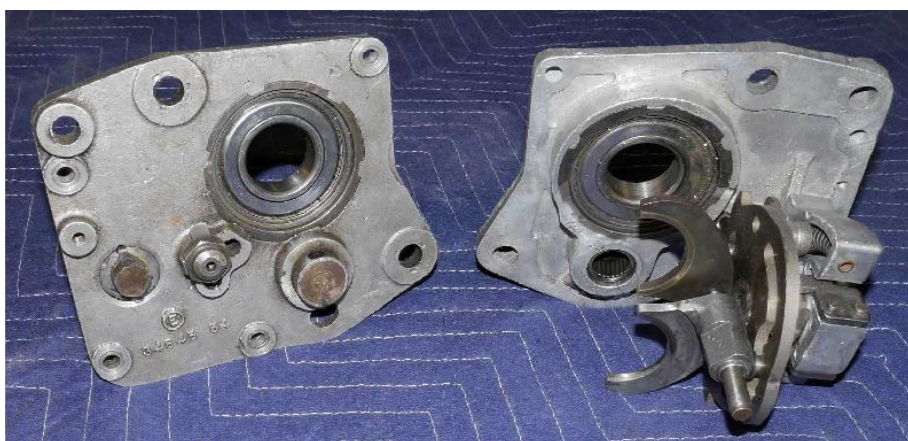
The Iron Sportster trap door assembly holds the mainshaft, countershaft, and shifter mechanism.
