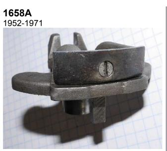
The countersunk screw is staked in to keep it in place.
