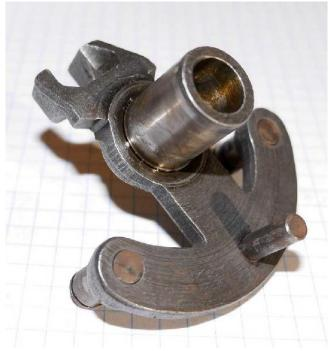
After 1971, the factory made this pressed-in pin a part of the carrier itself.
