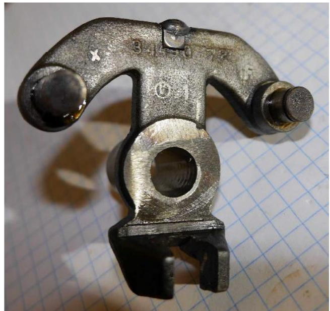
Some carriers have the 34490-72 casting part number on the "anchor". This one has a square pin like the -52 part. That means this is likely the -72 or -72A version of the part.
