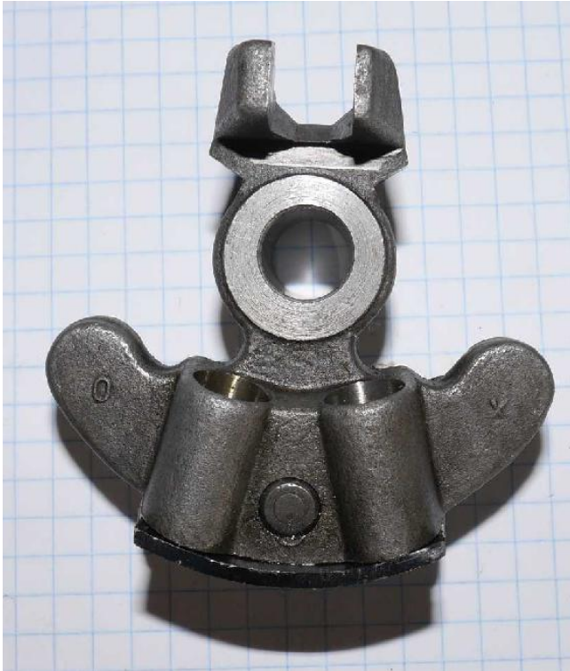
The early style carrier used plungers to ratchet the shifter plate.
