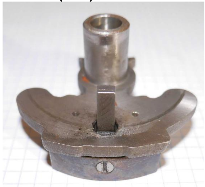
The early carrier has a retainer and screw.
