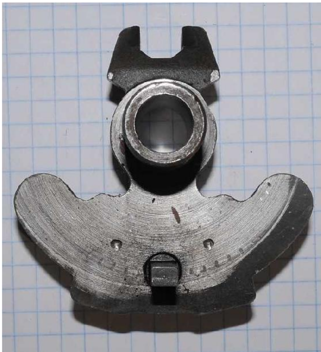
The side facing front has a square pin that sits between two springs.
