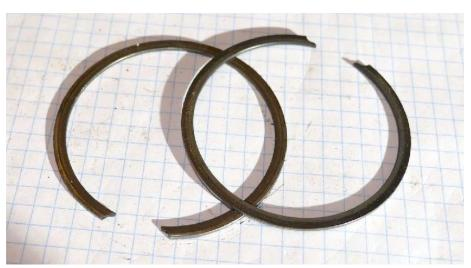
Sportster 35112-52 mainshaft roller bearing snap ring. The Iron Sportster takes two of these up until 1978, then one of these and one 11006 from 1979 to 1984.
