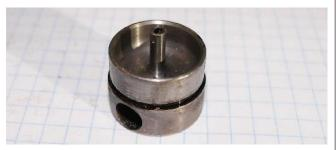
In 1973, in concert with moving the speedometer drive gear out of the transmission, the oiler was lengthened.
