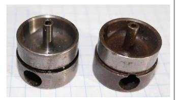
Two of the -73 parts, note cross hole is not accurately located.
