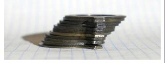
The washers stacked up. If there are gaps that means one or more washers are not dead flat, and you should find it and throw it away. The sound a washer makes when you plop it on a mirror or surface plate can also tell you if it flat.
