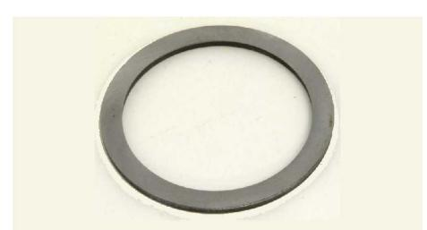
If you forget to put this in, you could seize the rear wheel at speed. Use Dr. Dick's trick-- put the tranny in without the rollers, then set the rollers, this washer and the snap ring from the outside.
