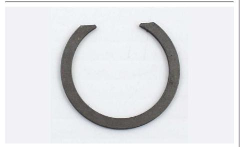
If you forget to put this in, you could seize the rear wheel at speed. Use Dr. Dick's trick-- put the tranny in without the rollers, then set the rollers, the washer and this snap ring from the outside. Use safety glasses.
