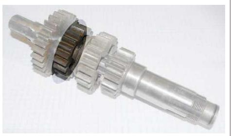
Mainshaft second gear is in the darker oval. Gears are named for carrying power, not the order on the shaft. The gears from left to right are mainshaft low, mainshaft 3rd, mainshaft 2nd, and the clutch gear.
