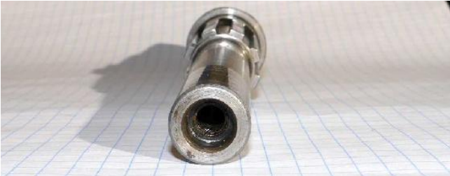
35044-56 has a hollow shaft.
