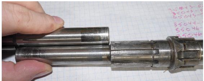
The 35046-71A mainshaft is not the early 35044-56 shaft without the hole. The late shaft is also a bit shorter.
