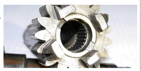
The mainshaft thrust washer left is pressed into the clutch gear. It captivates the Torrington bearing. This will set the spacing from the clutch gear dogs to the 2nd gear dogs.
