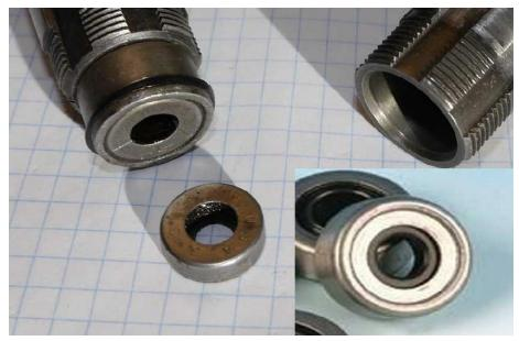
dry clutch electric start 37531-56B on left, near the early model dry-clutch gear with the extentison pressed in. The 12021 is on the right. It is bigger and goes directly in the electric start dry clutch gear above it.
