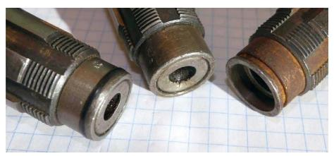
You press the extension into the early dry clutch gear. The one on the left has its O-ring and seal. The middle extension is a mystery since it is not grooved for an O-ring, it may be for early 1955 K-models.
