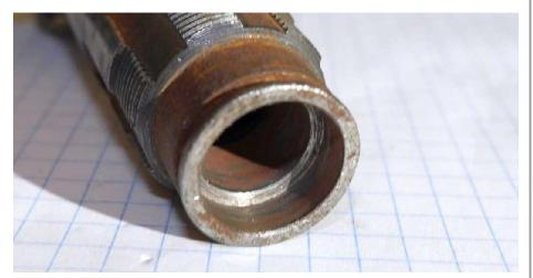
A close-up of the clutch gear extension without the seal or O-ring installed.
