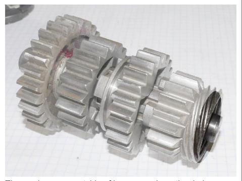
The washer goes outside of low gear, where the darker circle is in this picture.
