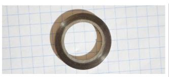
Countershaft thrust washer low gear right; 35818-72, 35327-73, 35819-72, 35328-73, 35821-72, 35329-73, 35820-52, 35821-52, 35824-52, 35825-52, 35828-52, 35829-52
