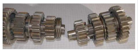
The left countershaft has a spiral gear as part of the low or 1st gear. It drives the speedometer on 1952 to 1972 models. The right countershaft is what would be used on 1973 to 1984 Iron Sportsters, the speedo is from the front wheel.
